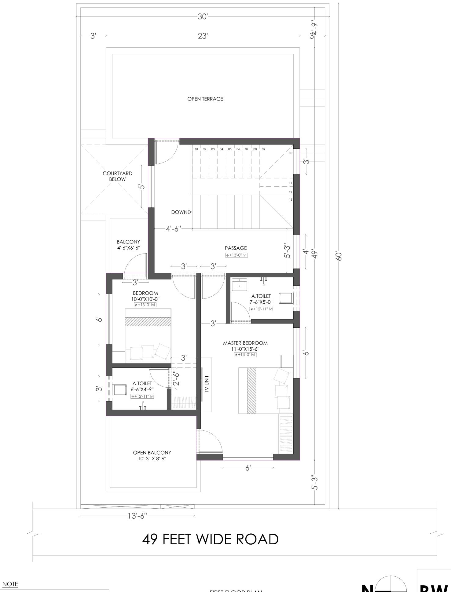
TOTAL BUILTUP AREA - 1871 SQ.FT FIRST FLOOR AREA- 743 SQ.FT FIRST FLOOR PLAN
